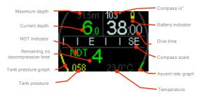
Fig. 22 Display NO decompression dive mode
